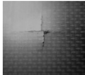
Fig.4 Impact damages in CFRP laminate.
