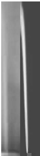
Fig.9 Flame behavior (V=5[m/s], OH mass fraction)
