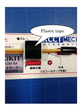
③ Wrap a rubber band around the plastic tape following to the photo below. Secondly, Put on a shortly cut plastic straw through the bamboo skewer
