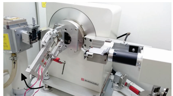
Fig. 11 Measurement of \sin^2\psi method
