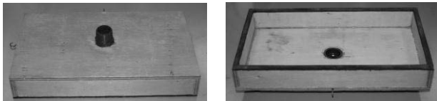
(a) Top view (b) Bottom view Fig.4 Geometry of floating-device of air-room type
