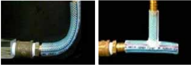
(a) elbow (b) T-shape elbow Fig. 5 Shape of test section (polyvinyl chloride)
